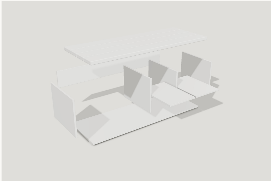
Every part, exploded: bottom, 2 sides, 2 dividers, 2 shelves, back rail, 4 seat boards
